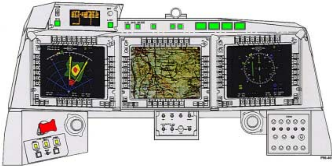
Figure 2. Rotorcraft Pilot's Associate (RPA) advanced technology demonstration aircraft cockpit with three 12-in. active matrix liquid crystal displays (AMLCDs) and virtually no electromechanical instruments. Cockpit designed in 1990s, built 1998, flown as non-operational engineering program (one aircraft) to learn how to use advanced electronics to significantly reduce combat crew workload. The total information carrying capacity of this research cockpit is twice that of the F-22A.
