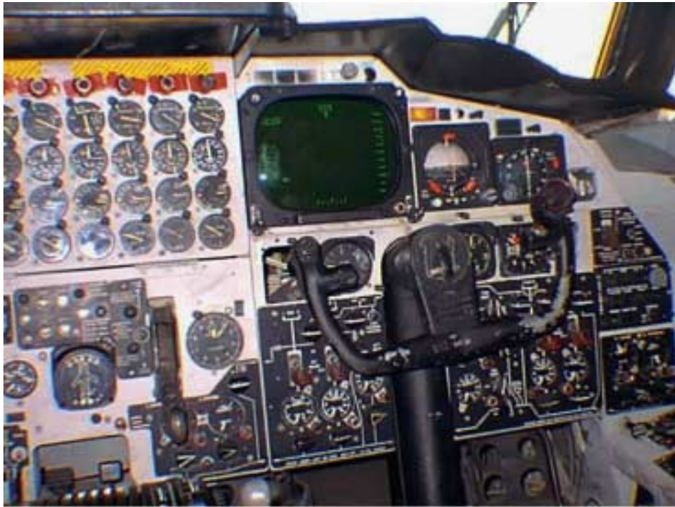
Figure 1. B-52H pilot main instrument panel with one electronic display (9-in. monochrome CRT) plus some 60 electromechanical instruments. Cockpit designed in 1950s, built 1960-62. The Air Force plans to operate B-52s until 2046. Note closable screen for nuclear flash and synthetic vision for low level flight (LLTV or FLIR image displayed on CRT)
