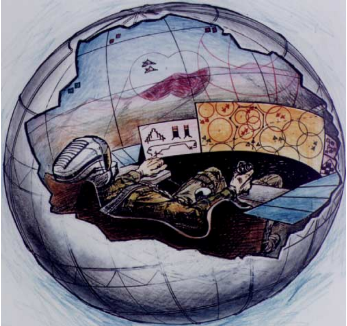
Figure 6. Concept for 2020: Immersive Cockpit . Encapsulated crewspace realized via combination of direct-view, projection and head-mounted displays.
